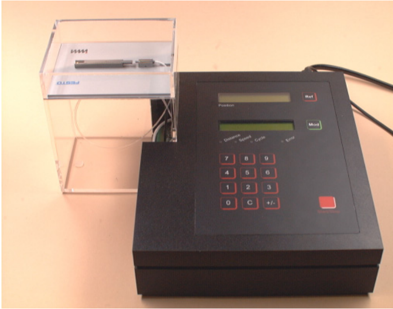
Figure 3: Freely programmable control of the stage
