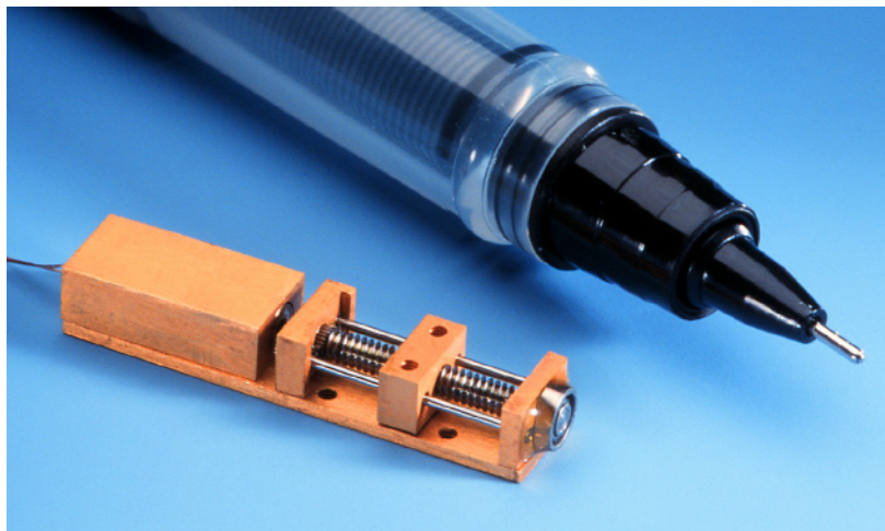
Figure 4: Open loop controlled linear stage compared to a pencil
