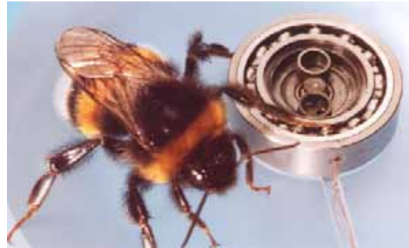
Fig. 14: Ultra flat micro drive system
