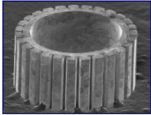
Fig. 14: optimized tothing of the planetary gear wheel
